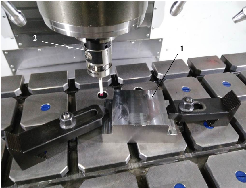
Fig. 4. Measurement of workpiece control points
